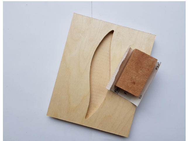
Figure 4. Sanding the edges of the main body
